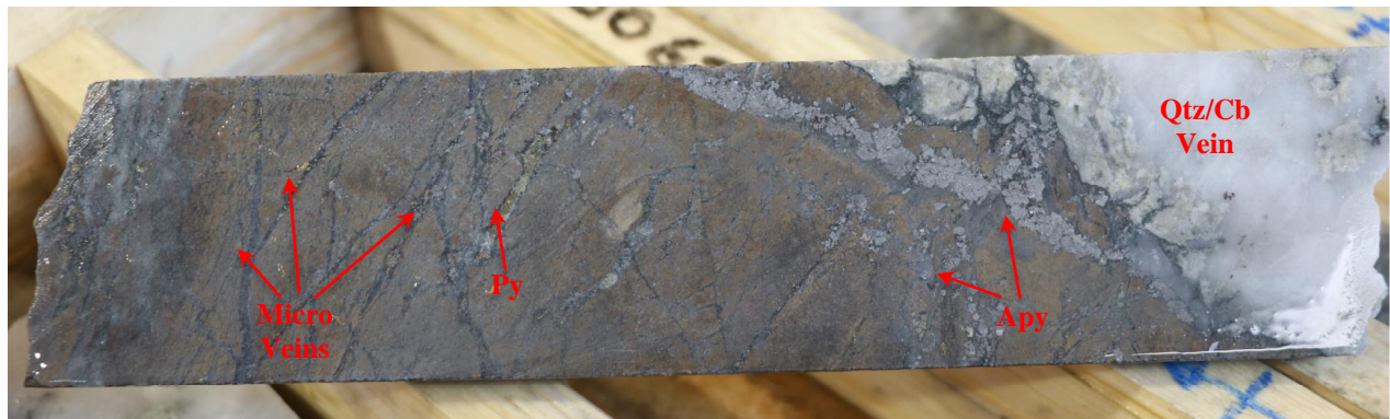
Figure 3. Example of mineralised core from hole FAVD0062 (from 225 metres downhole grading 8.8g/t gold), highlighting a zone of pervasive albite alteration with polyphase quartz and quartz-carbonate (Qtz/Cb) veining and associated arsenopyrite (Apy) and subordinate pyrite (Py)
