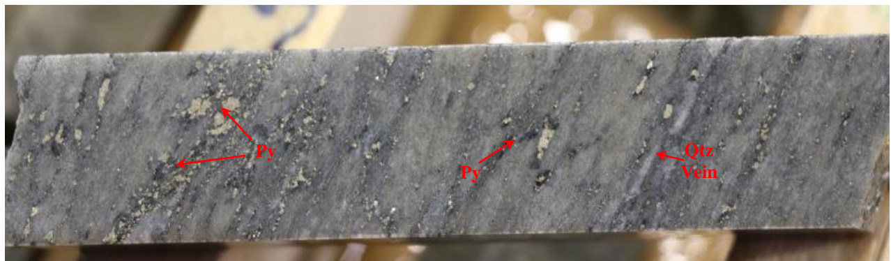
Figure 4. Example of mineralised core from hole FAVD0064 (from 200.8m downhole grading 73.6g/t gold), highlighting a zone of intense foliation and textural destruction with strong sericite-silica alteration, thin wispy quartz (Qtz) micro-veinlets and strongly disseminated pyrite (Py)
